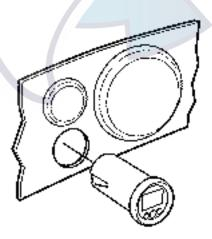
Drill a 2 1/8" diameter hole using a hole saw and hand drill. This is a standard hole saw readily available for rental or purchase. Or, any marine service shop can handle this task.
