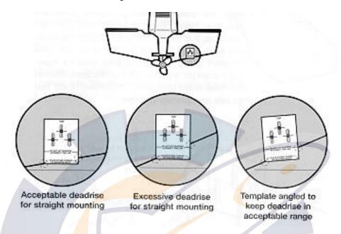
Using a pencil or punch, mark the three mounting holes onto the transom.
